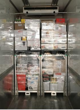
SpaceInvader doubled-stacked pallet racks lined up in terminal - and in truck before departure. ASKO Hedmark, Central Norway
