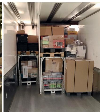
Maximum height with double stacking during transport
